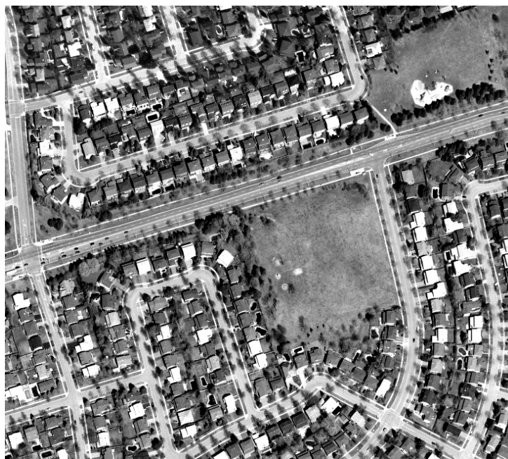
Figure 8. Reverse-lot subdivisions. Houses line an arterial street but can only be accessed by internal subdivision streets. The example is York Mills Rd. near Leslie St. and shows the RCS with locals, collectors, and arterials used to organize the street system and housing areas (J.D. Barnes First Base Solutions, 2002, ORTH176310484502002FBS).
